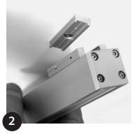
Move sliders on MOMO-L Power base to match plate spacing. Lock slider in position (grub screw/hex key).
